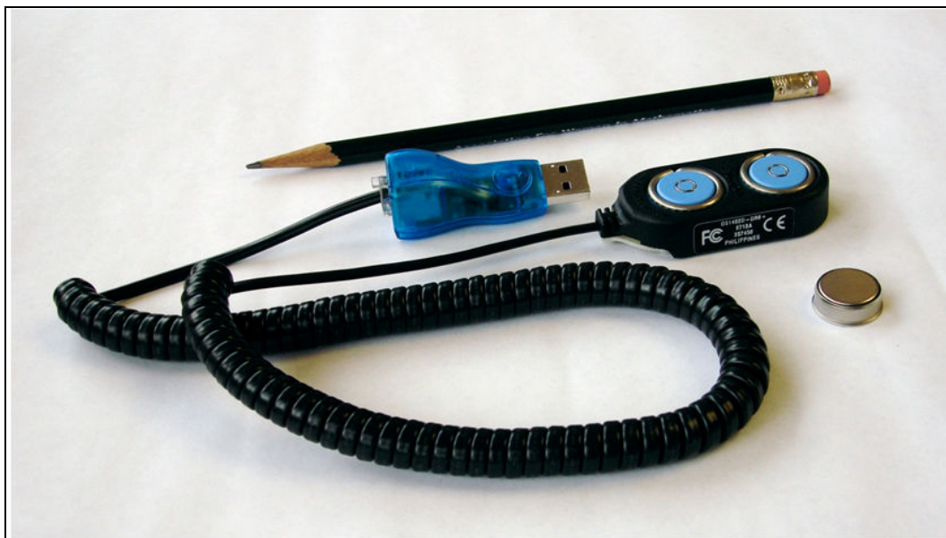
Fig. 1. DS1912G iButton and the RFID reading device.
