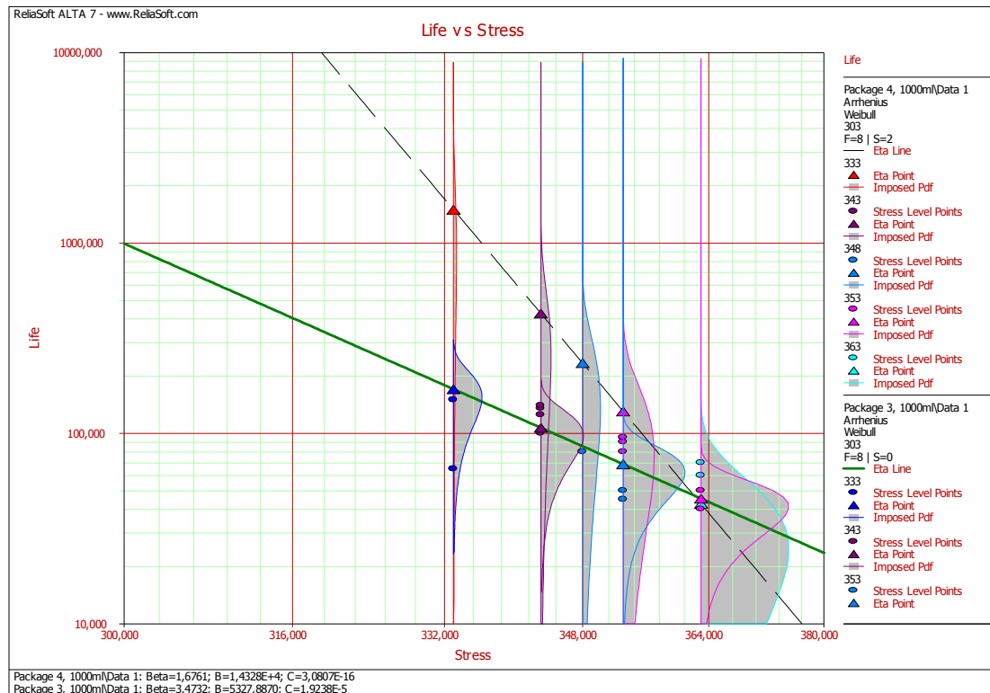
Fig. 11. Life stress analysis: Pack 3 vs pack 4. Glass bottles 1000 ml.
