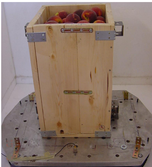
Fig. 4. Simulation of intra-farming transports of peaches by means on an electro-dynamic shaker (Ragni et al., 2001).
