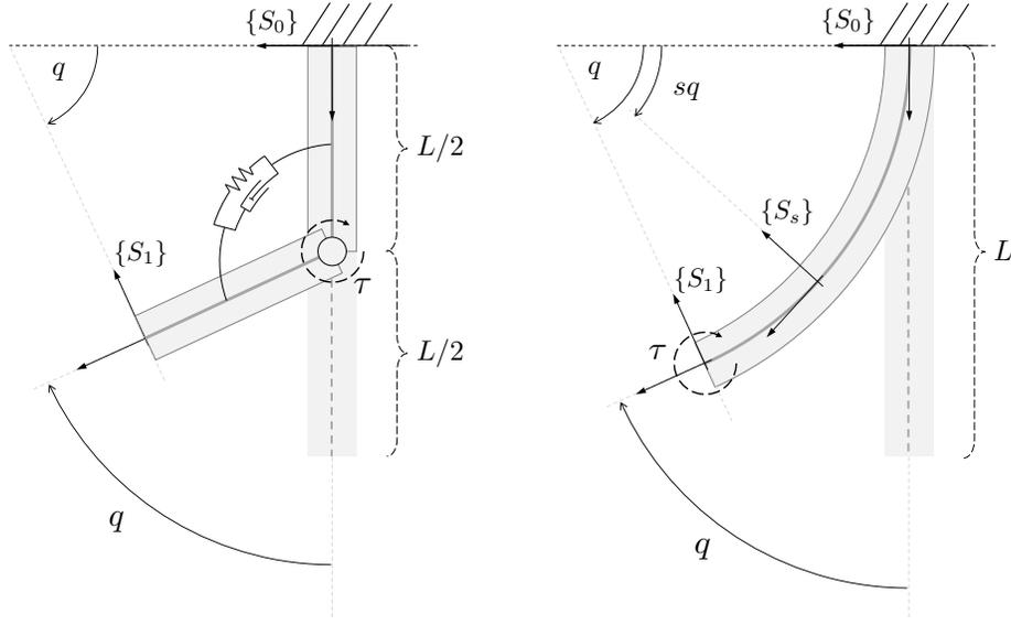
Figure 8: A constant curvature segment together with and lumped rigid-link model serving as its first order approximation. The two resulting dynamics have equivalent structural properties, but are described by substantially different dynamic equations.
