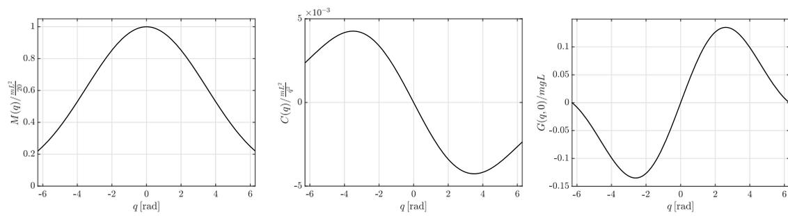
Figure 10: Evolutions of (46), (47), and (49) all normalized w.r.t. the quantities that appear linearly in their expression. A change in those quantities result in a linear scaling of the plots along the vertical axis.
